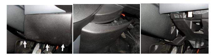
The trim on the left of the steering wheel is held on with 4 torx screws, 2 are on the underside, the other two are visable behind the speedo surround and the trim piece i.e. Piano Black..
