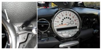
Starting not to remove the colour line trims the passenger side is held on with 5 torx screws, two of these are visible behind the air vent we removed and behind the Speedo surround we just removed, the other 3 screws are under the trim, so just open the glove box and these will be visible..
