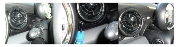
The next job is to remove the Speedo surround (not as daunting as it may seem), this is also held in place by 6 torx screws, two of these are hidden behind the air vent at the top of the dashboard, two behind the plastic cover we removed in step one and two behind the trim behind the steering wheel, it's not necessary to disconnect the surround from the hazard lights, just turn it around and sit it on top of the dash..
