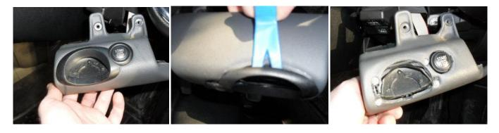
My only advice on the above would be that the plastic key slot surround is very fragile, I have ordered a replacement part from me dealer as mine broke when removing it. The part number is 51452753776 and costs about £7 from MINI.
