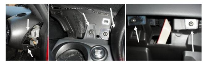
The final part of the process involves removing the ignition/key slot from the trim, this involves removing the plastic trim cover. To do this use one of the plastic trims and prise it off at one side, using a small allen key press the visable metal clip to release the cover, the same process can be used for the other side. Once you remove this you need to unscrew the key slot, this is held in place with 4 T10 Torx screws..
