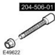
Halfshaft installer adapter 204-506-01
