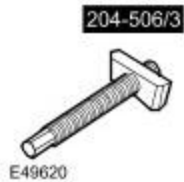
Halfshaft remover/replacer 204-506/3 (LRT-60-030/3)
