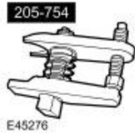
Ball joint separator 205-754 (LRT-54-027)
