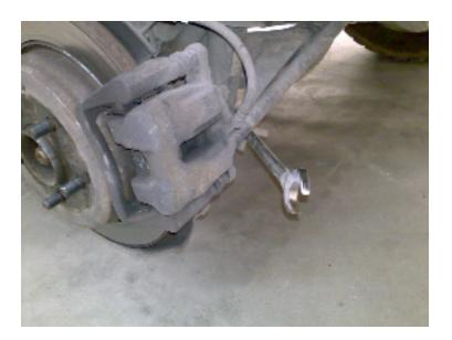
On the opposite side place another spanner on the nut head. I used a socket here. Release and remove the pin. It might need a tap of a mallet to help it through.
