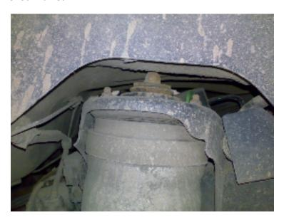
**Below:**Release the air from the airspring by slowly loosening the airline feed (green pipe) with a 12 mm open ended spanner.It's a slow job as you don't get much room to use the spanner.Before you do this, it's advisable that you clean the top of the turret to avoid any dirt entering the airspring
