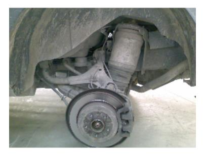
**Remove Plastics**:In the following order, remove mudguard 3 X screws, remove wheelarch liner 3 screws and approx 4 plastic rivets, remove wheelarch eyebrow.
