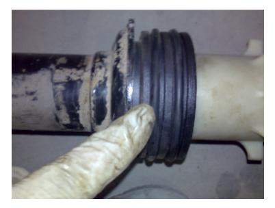
Slide the airbag down over the new spindle aligning the tab with the little metal checkout that you should have marked or made note of its position earlier. It wont go fully back down into position I'll describe how to do this later , just make sure they're aligned for now.
