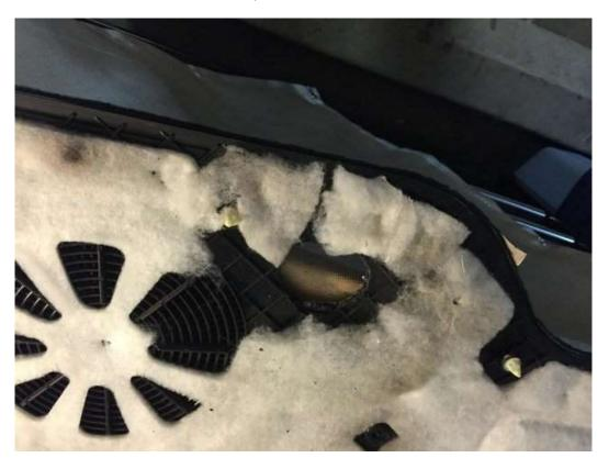
15. Test fit. This is the part where I actually determined that 14mm height was needed for the tabs. my original calculation put it at 17.5mm but at that height the handle didn't countersink into the carpet the way I needed. I also took this time to make sure that the tabs were all bent perfectly to grip the edges of the inserted handle.
