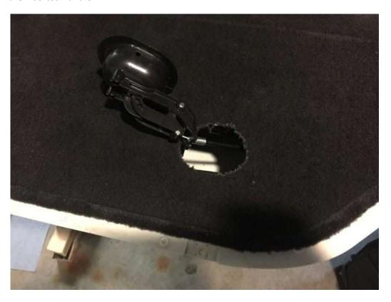
16. Getting close. Just making sure that everything fits and looks factory. once I was satisfied here i used a center punch to mark the hold position for the mounting screws on the top and bottom of the handle assembly. I then drilled out the holes with a 1/8" bit, then used #8 self tapping screws to create the thread. In final assembly, I used #8 3/4" black automotive screws so that they would blend in.
