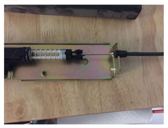
4. Fix actuator clip with zipties. This is a preliminary fix. This will solve most problems with the actuator separating from the cable, but will not prevent issues related to the actuator or a dead battery.
