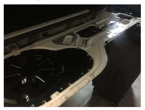
3. Remove the Rear actuator assembly (8mm bolts) and the plastic cover of the actuator assembly (T15 Torx). Here is the biggest culprit. The black plastic clips can break causing the cable to fall loose from the actuator.
