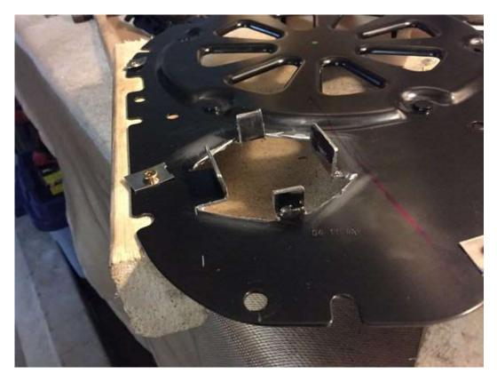
10. Moving on to the actuator assembly, I needed a point where I could attach this secondary pull. I wanted to make sure that the new handle would be functional for any possible failure, so "sistering" the new cable to the existing one was a must. I used a small scrap of sheet metal cut into a triangle, then drilled a hole in it for the new cable and crimped it tightly to the existing cable. This setup also helps to reduce any lateral stress on the actuator when you pull the auxiliary cable.
