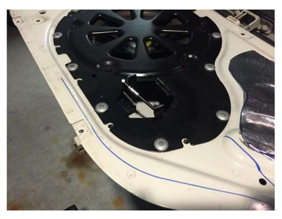
14. Use a dremel to cut a hole in the carpet section of the tail gate using the center point we drilled earlier. Be sure to remove the insulation behind where you are going to cut FIRST or it will bind up. You will need to remove some extra plastic material at the N S E W positions to make clearance for the metal tabs. Do not remove more than 2mm or it may be visible after the handle is installed.
