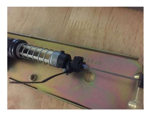
5. Buy Cable pull handle. I searched forever to find something just right. I looked at tailgate handles, bike brake levers, hood releases, mower throttle cables, car door handles, Discovery I rear gate handles, etc. All of them were either too expensive or wouldn't have looked right countersunk into the LR3's rear carpet. Then I stubled across these pull cables for recliners. PERFECT!
