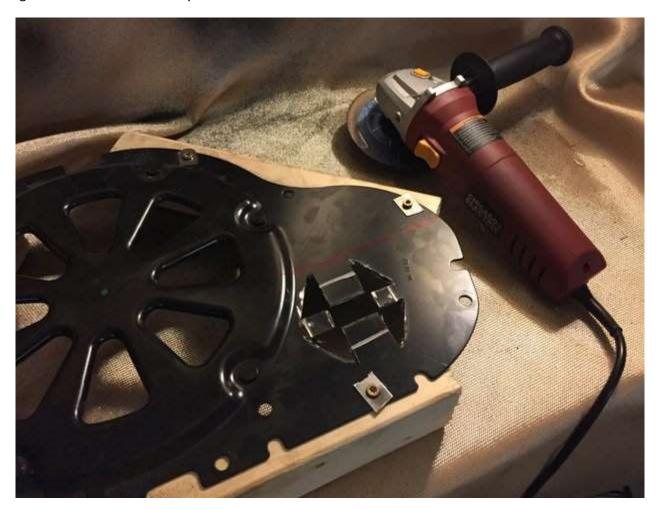
9. I scored the surface of the metal to create a natural place for the 90 degree bends, then used a pliers to bend up the prongs. Once this was done, I used a grinding disk to make sure that the top edge of the prongs was aligned and flat. Using a caliper I measured the thinness required from the subwoofer mounting plate to the carpeted gate and determined the prongs needed to be about 14mm tall.
