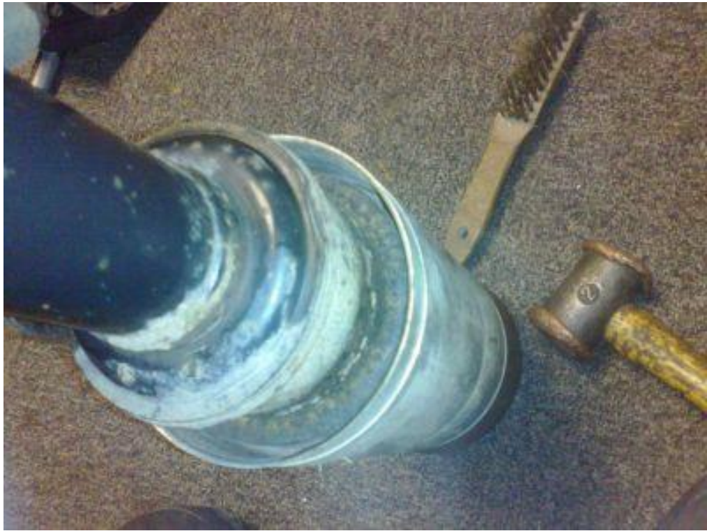
I found they came out when tipped the spring upside down and gave it a knock with a hammer
