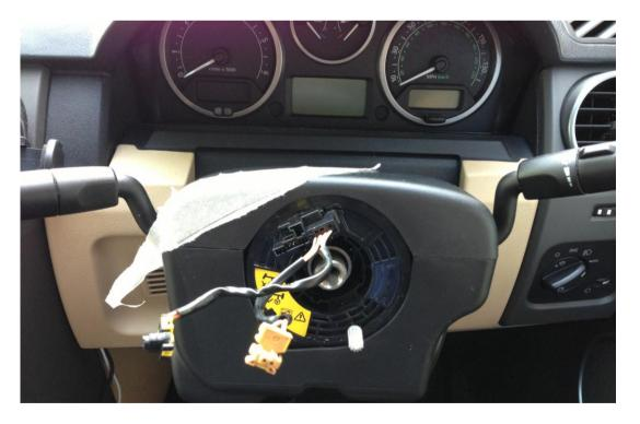
Make sure you take note now on how the clock spring is located – grey lug bottom slightly to the right and the block where the connectors are at the top and slightly to the left. It's important to note this to make sure you put the new one on located in the same way.
