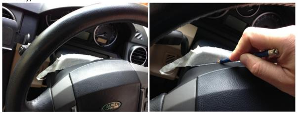
Remove airbag – You can by a tool, but like many, I made my own using a coat hanger, or the metal part of it anyway. You need a hook on the end about 5mm long. I had a longer hook the other end for me to pull on to release the airbag, which worked fine for me:
