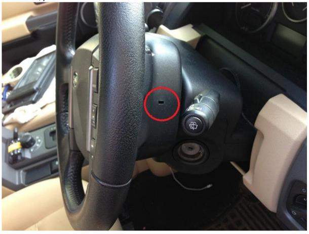
Once you can feel it hooked on, give it a pull and the airbag will start to pop out from the steering wheel. Does take a bit of force so don't worry if it's not coming free... may need a bit more of a tug. Take the tool back out and repeat on the other side. The airbag should now release more and you can just gently
