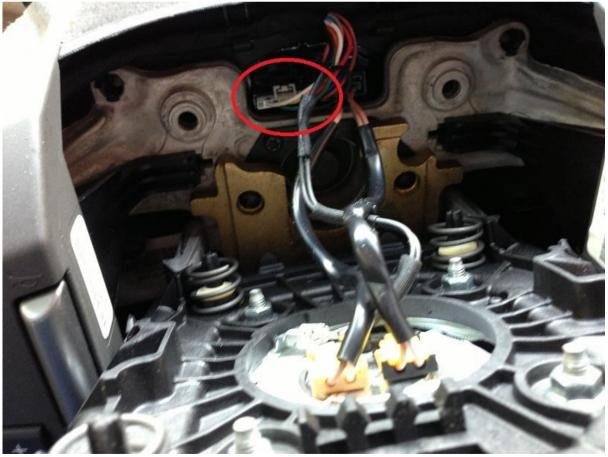
Now to remove the steering wheel. Use a 16mm socket to remove the bolt, undoing counter clockwise as normal. Tip – to avoid pulling the wheel off too hard and suffering from a 'steering wheel in the face, don't remove the bolt completely until you have pulled away the steering wheel from the
