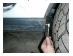
Remove the 7 trim clips from the underside of the plastic sill. (trim removal tools)
