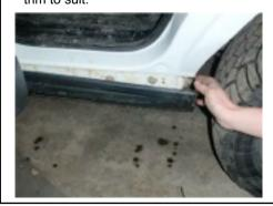
4. Find the hole on the inside of the chassis leg.
