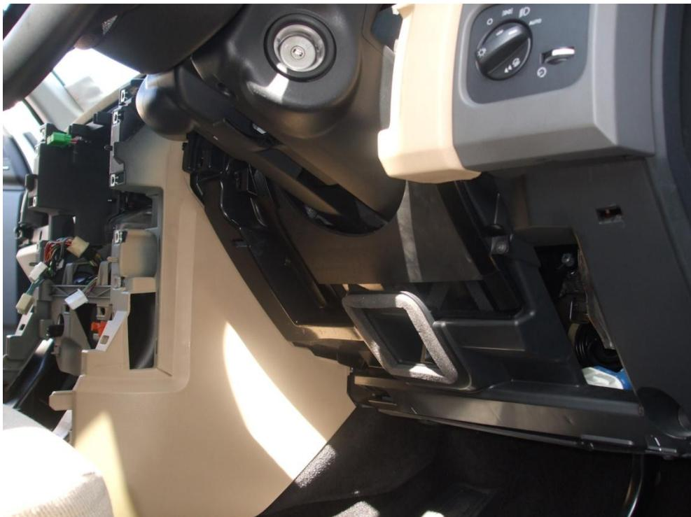
22. Squeeze the stays on either side of the lower glovebox when open, so it drops down to its lowest position.
