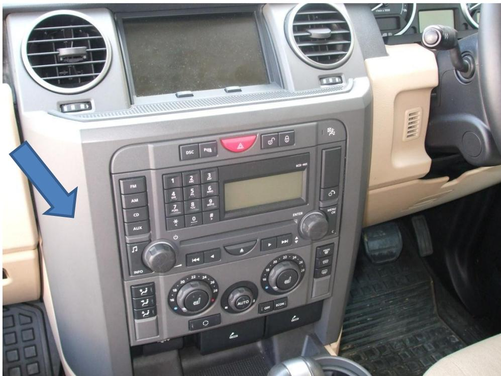
5. Remove the sat nav, stereo, heater controls etc. Be careful of some of the connections at the rear, especially the optic fibre ones. Note that the bottom one, the ashtray and 12v sockets, won't come out yet.
