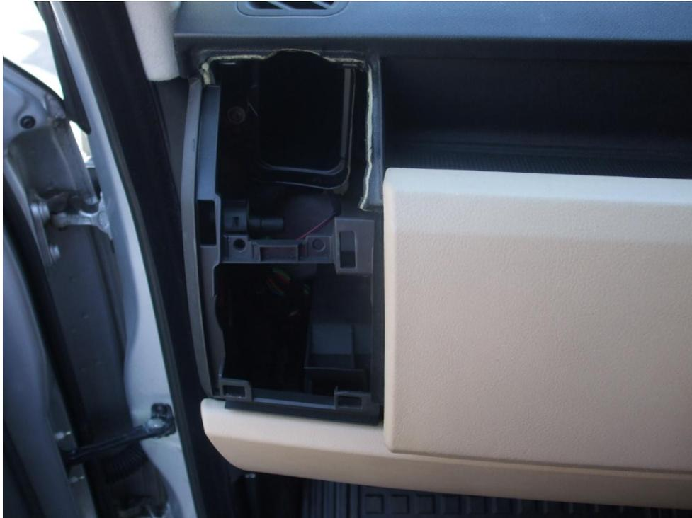
7. Remove the inner bit of the upper glovebox. There's two spring clips on either side, located where the arrows are. This was a real pain for me and I thought it was going to break; careful use of a screwdriver to prise it off was needed, plus pushing from behind (explains why the vent had to be removed first). The hole in the bottom centre takes a plastic clip from the inner lining, it seems to stop it coming out easily.
