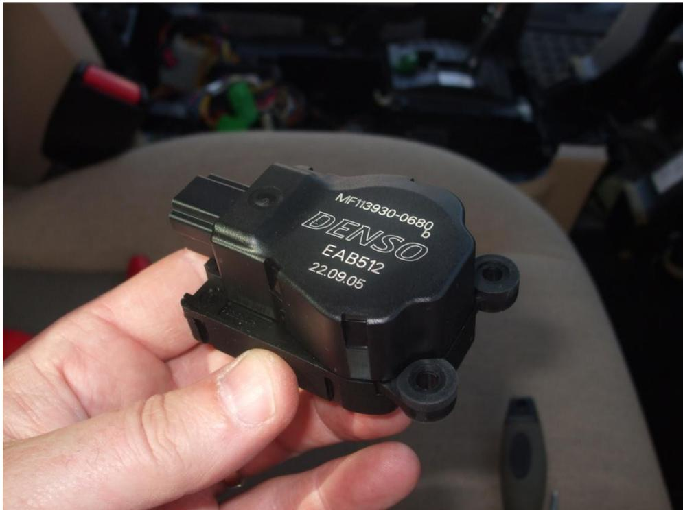
26. From what I found out by trial and error, there's four of these little fellas hiding away. There are two on the left (passenger side) – the bottom one (big arrow) does the passenger side temperature mix, the top one controls the air flow between the footwell and the face vents.
