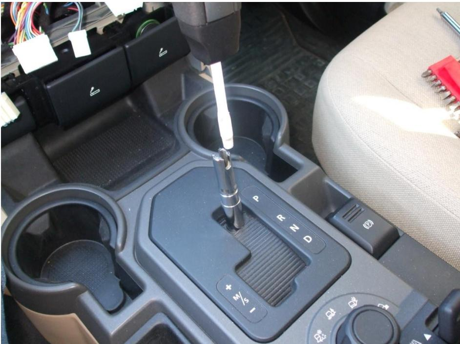
14. Remove the Torx screw from just in front the EPB handle.
