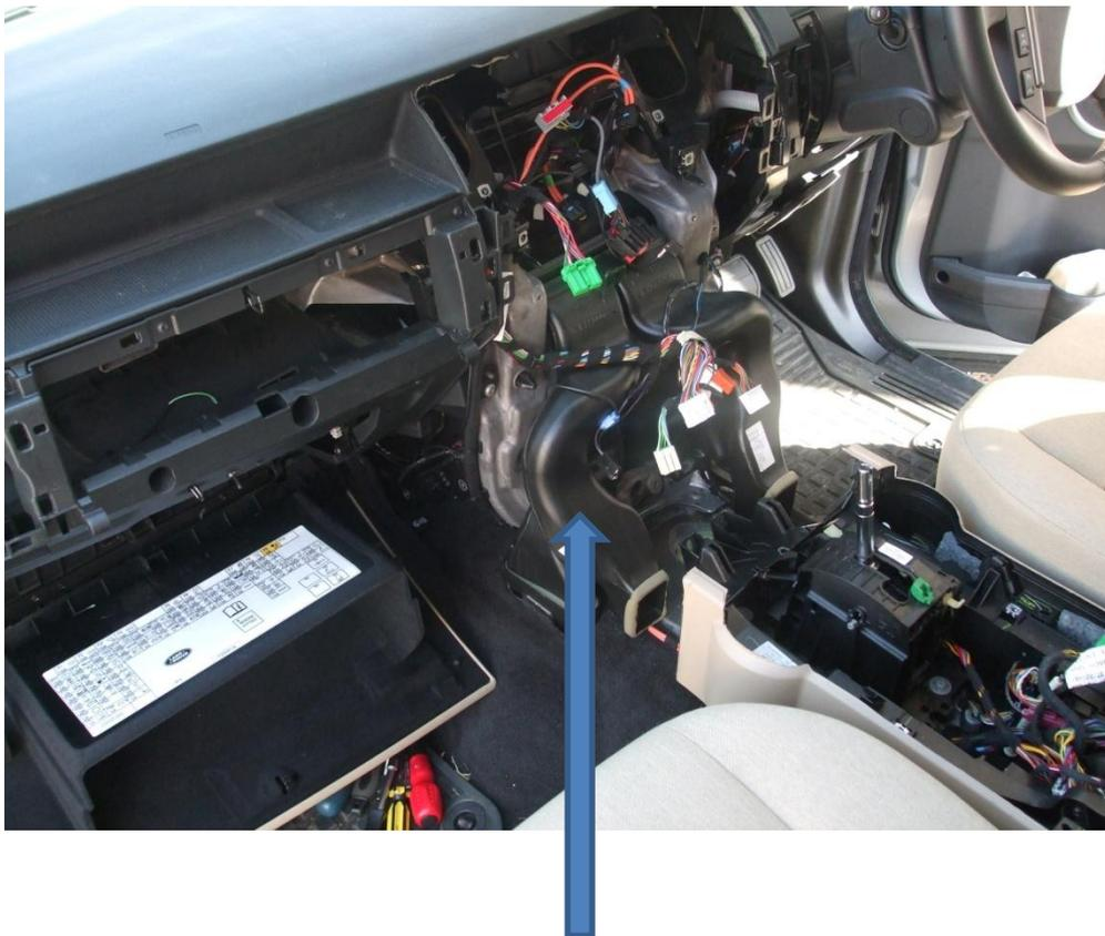
Here's the plastic ducting I referred to in point 23.
