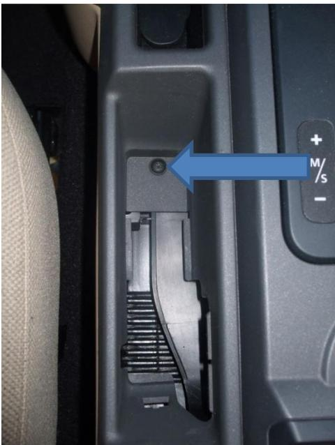
Now pullwards up the top section of the console. A lot of plastic breaking sounds will be made that sound expensive. At least one clip of mine is permanently broken. I don't think there's any trick here, just luck.
