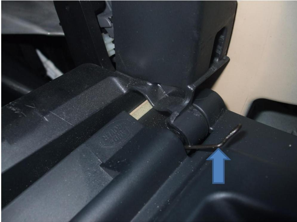
10. Looking inside (where the satnav once was), find the mechanism that dampens the opening of the glovebox door. Move it to a point where you can see as shown below (the pin won't be half out... you need to do this) and push it from the left-hand side with a small screwdriver etc. Don't push out too far or else it's goodbye pin. Pull out the remainder of the way with long-nose pliers.
