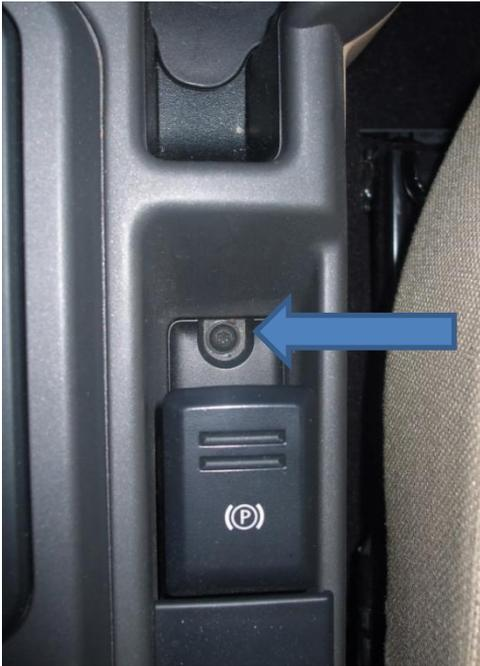
15. Remove the rubber sunglasses holder, then the plastic bit underneath it. A hidden Torx screw should be found underneath. Very cunning Mr Land Rover.
