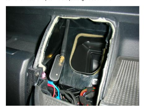
Have now moved the LED from the GSM to much better place than stuck behind the dash, I just cut the led from the pcb and stuck a length of wire on it, I have placed it on the centre pull off dash panel at the left hand side near to the cigar lighter, it can be seen easy from the driving position and not be in your driving view.. Also moved the fuse to under the pull of panel under the steering wheel for better access.
