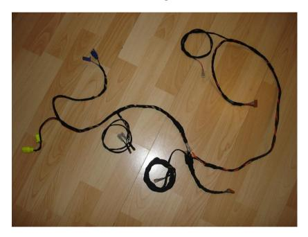
Having had just the GSM unit wired in temporarily for the last few weeks, I have finally finished off my conversion of the harness to what I think should have been for a very nearly plug-and-play D3 installation with the two control modules installed behind the lower glove box.
