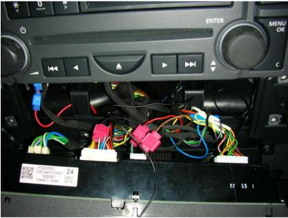
The red wire at the back with the blue scotch lock on is the feed from the cigar lighter. this is the wire that the red and white & the orange wire connect to.
