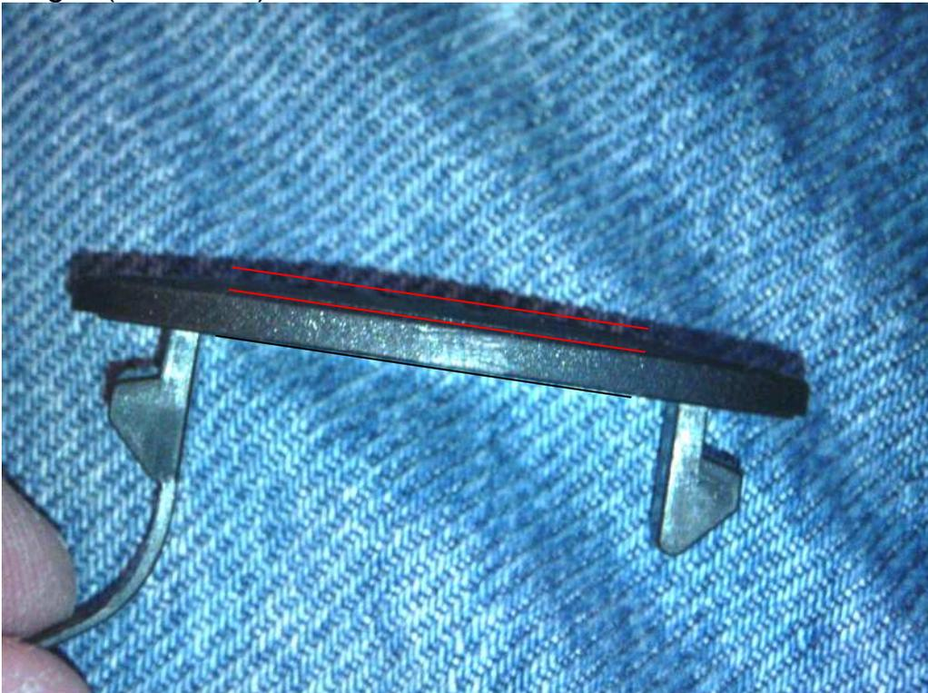
Next you need to reduce that material down in the exact shape of the new shiny bit. In fact about 0.5mm less to ensure a tight fit.
