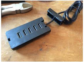
You can see that the whole board is just screwed in by 4 screws, so I'll get another one for the rear cubby and will do away with the case possibly. You could also solder wires to the Pos and Neg points on the back of the board to make the wires tidier by not coming out of the side.
