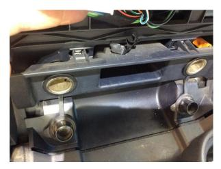
Unclip the connector for the 12v socket
