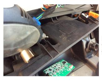
I then used a dremmel to do a simple hole for the cable (cut the plug off the end of the cable) You can feed the end of the cable through the back of the plastic and through to the 12v socket.
