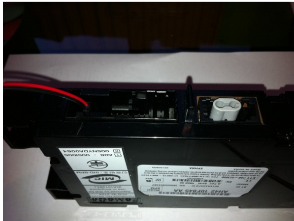
The 2 pin end fits in the new Bluetooth module
